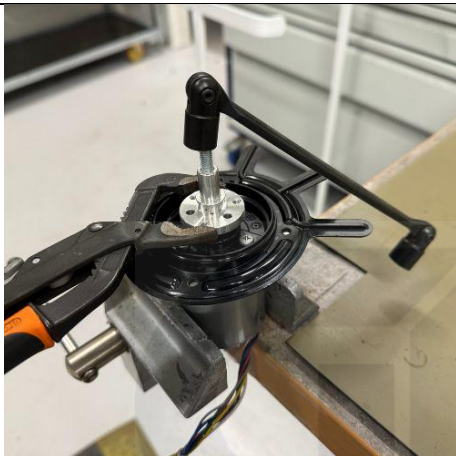
Step 3: Hold the hub with locking pliers (e.g., a multigrip). Use a 10 mm wrench on the bolt and tighten it — this will push the hub upward and release it from the shaft.
