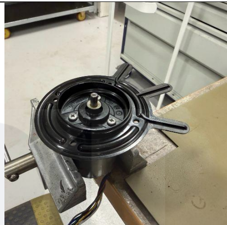
Step 4: Remove the three screws that hold the cutting motor plate.
