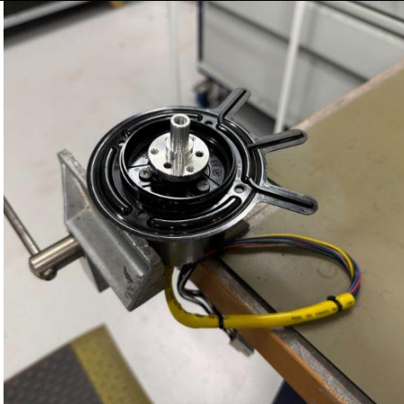
Step 1: Secure the cutting motor firmly in a bench vise.
